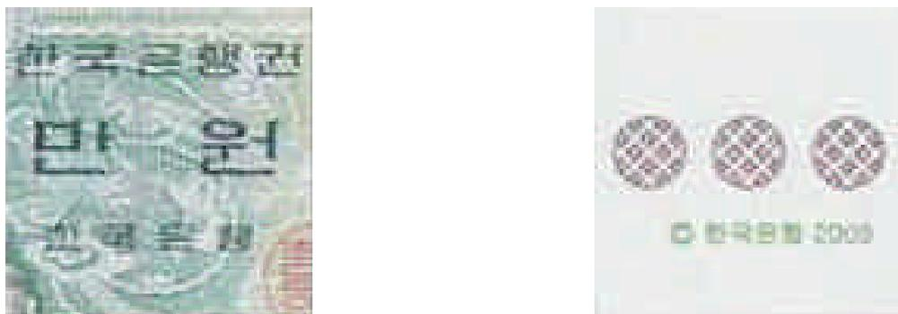
Figure 7 – Bank of Korea 10,000 Won note: Internet illustration of 99 x 101 pixel details of windowed thread (left) and optically variable ink (right).
