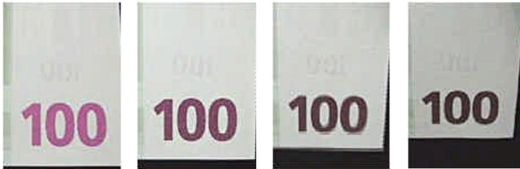
Figure 15 – European Central Bank: 4 movie frames (107 x 152 pixels) of a tilted OVI feature on a euro 100 note: the OVI print in the movie shifts from bright magenta to dark brown, while the actual color shift is from magenta over gold to green, when correctly displayed.
