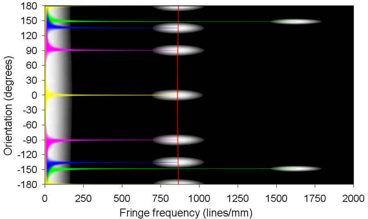
Figure 5 – Orientation-frequency analysis (OF-diagram): orientation versus fringe frequency by unwrapping the diffraction pattern of Figure 4.
