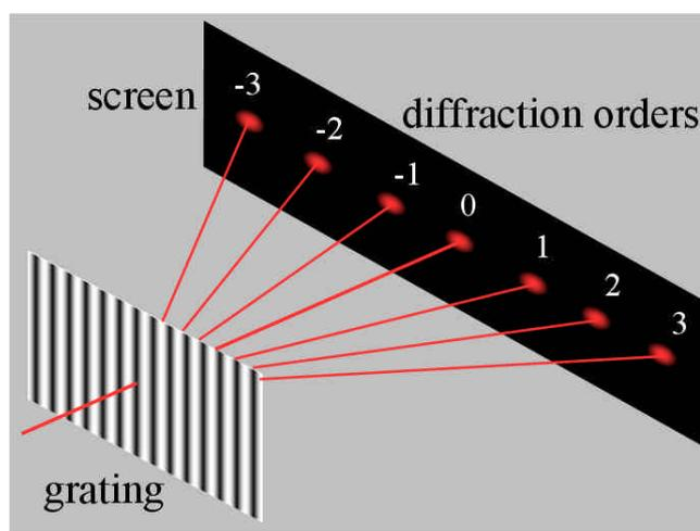
Figure 1 – Schematic illustration of the diffraction of a monochromatic light beam by a grating into a zero order and higher orders. The fringe frequency is not to scale but amounts hundreds to thousands of fringes per mm.
