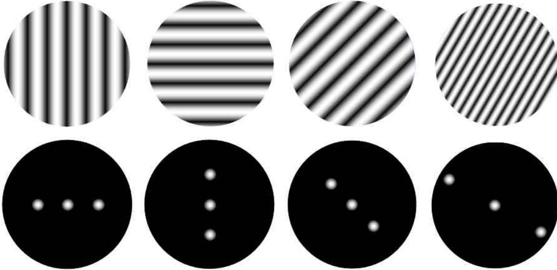
Figure 3 – The relation between grating parameters (top) and the pattern of the diffracted orders (bottom). Only the zero order and both first orders are shown. The light source is monochromatic.
