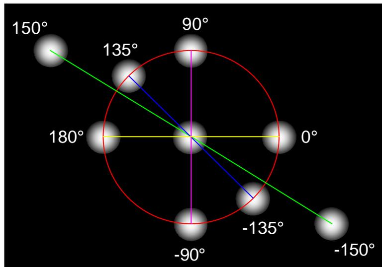
Figure 4 – Combined diffraction pattern of a DOVID composed of the gratings shown in Figure 3.
