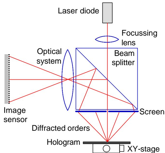
Figure 6 – Possible optical set-up of the laser scanning unit of a Universal Hologram Scanner.
