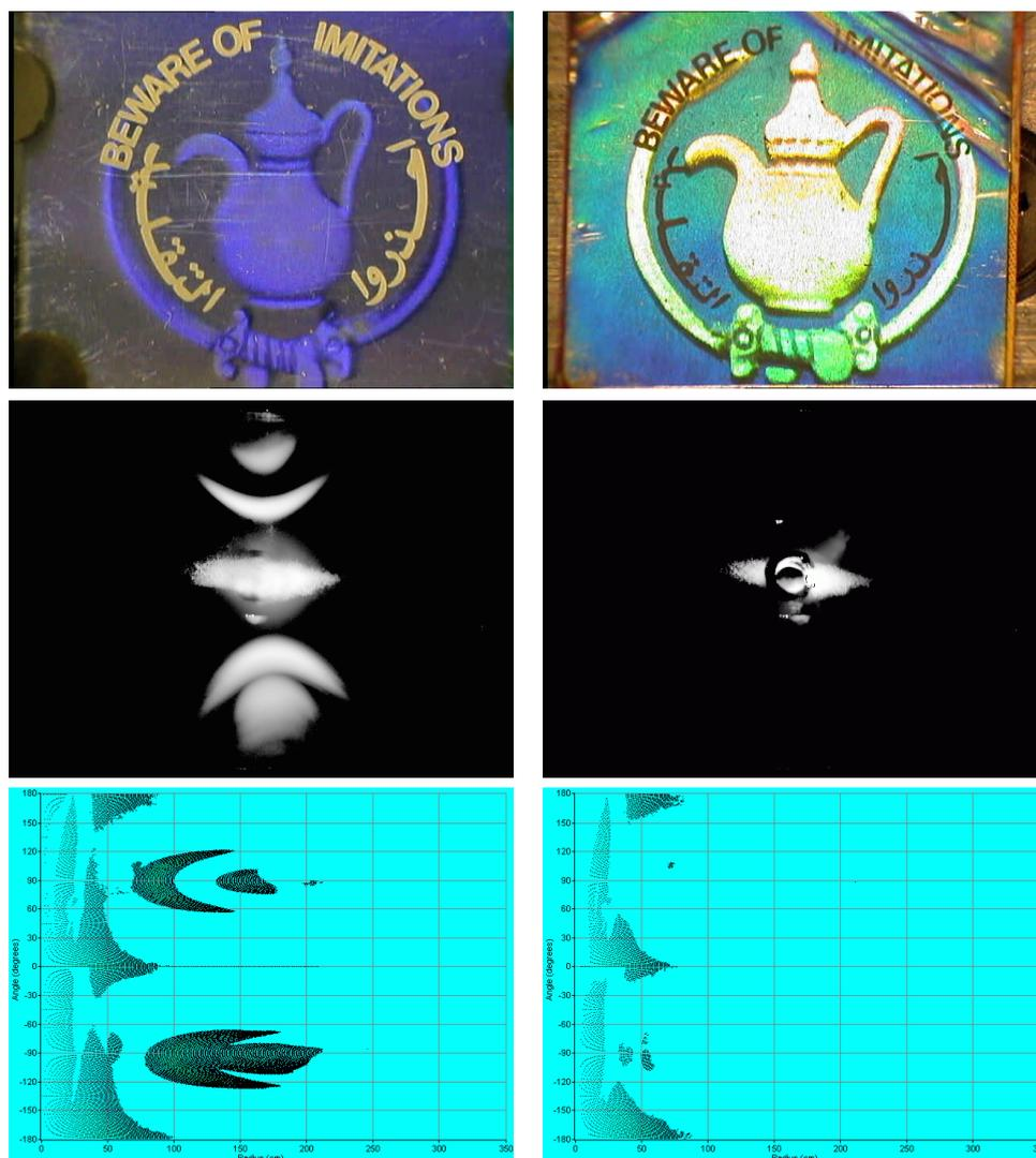
Figure 8 – “Coffeepot” holograms: original (top left) and counterfeit (top right), their diffraction patterns inclusive zero order noise (center) and their OF-diagrams (bottom).
