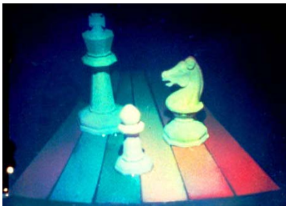
Figure 8 – “Chessmen” the first true-color, one step, white light transmission rainbow hologram made in 1979 by Steve Benton, William Houde-Walter and Herbert Mingace Jr. of Polaroid Corporation. Hologram size 4 x 5 inch.
