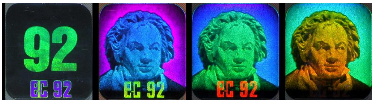
Figure 7 – A four-channel multicolor rainbow hologram of a tiny model of Beethoven’s head on the 1992 Eurocard, photographed at 4 different angles while rotated about a horizontal axis. No changes in vertical parallax are observed, but the color of the separate image elements change with the vertical angle of observation. Hologram size 15 x 17 mm.
