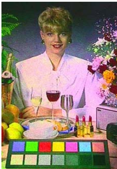
Figure 9 – True-color hologram by Light Impressions, produced in the late 1980s or early 1990s. Because the hologram is made using RGB color separation films, it does not display in three dimensions and is actually a 2D “in-plane hologram”. Hologram size 110 x 130 mm.
