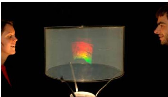
Figure 11 – Example of a 360° cylindrical holographic stereogram. Hologram size 10 x 50 inches, 40 cm diameter.
